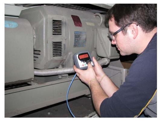
The SM-Keypad Plus pictured above is a low cost tool that should be in the toolkit of every technician dealing with Control Techniques AC drives. It offers the following abilities:
